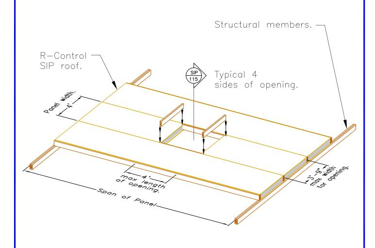
Note: For openings bigger in size than shown above or for openings that cut through splines, provide additional framing to support panel edges. This additional framing is to be located under the panels and framed into the main structural members.
