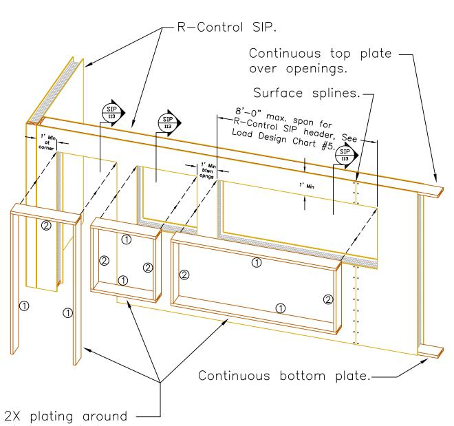
2X plating around window and door openings. Numbers indicate sequencing for installation. Refer to SIP-115 for connection of 2X's to OSB facings.
